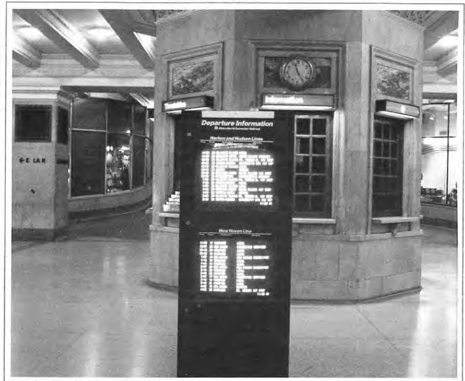
Fig. 4: One of the ten public video monitors placed strategically throughout the terminal, each with a separate screen for New Haven trains. Other monitors, for railroad personnel only, display train information in real time rather than scheduled time.
