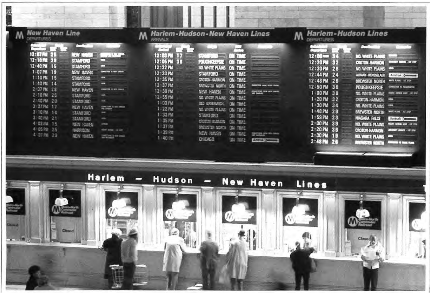
Fig. 1: Omega Board installed in the main concourse of Grand Central Terminal. A traditional split-flap design in keeping with the building's landmark status conceals sophisticated display electronics.
